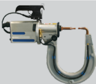
C-Tong 350mm throat depth, water-cooled
